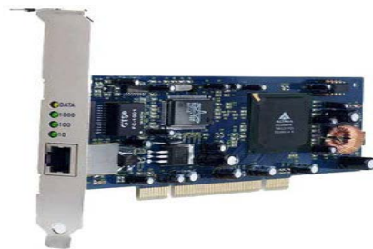
Gambar 2.1 Network Interface Card (NIC) / Kartu Jaringan
